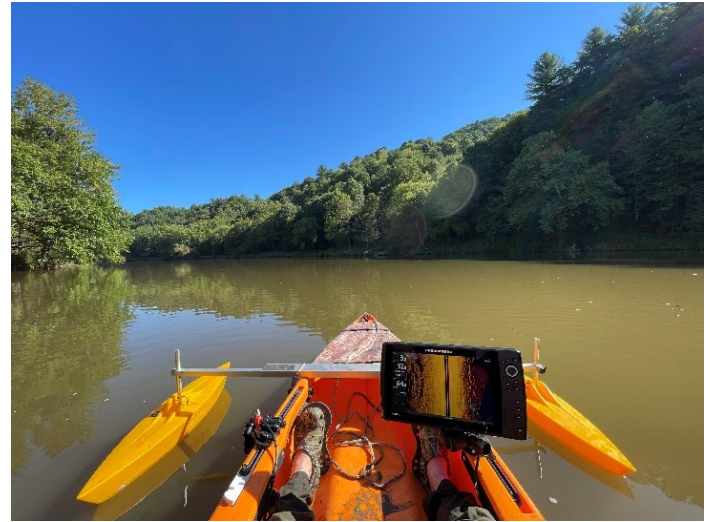
Taken on the New River, this photograph shows the VDHR team at work documenting areas above historic dams that may have inundated cultural features such as fish weirs. A small side imaging unit is kayak-deployable to scan the most remote areas.
