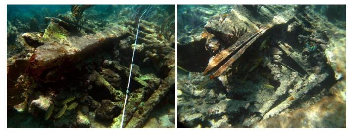
The south end of the metal wreck showing the keel assembly and attached frames. Left, prior to the storm the keel appears to be a single metal beam; right, after the storm the laminated nature of the assembly is evident.
