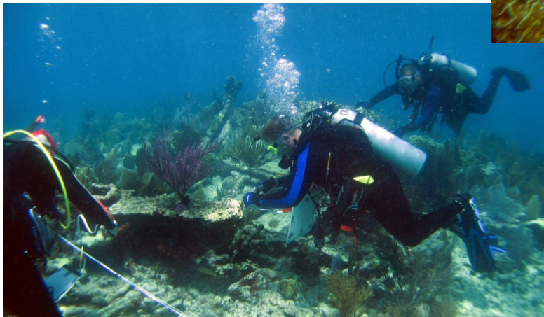
Per Kistler and Erik Kistler using trilateration mapping to record features on Pickles Reef.
